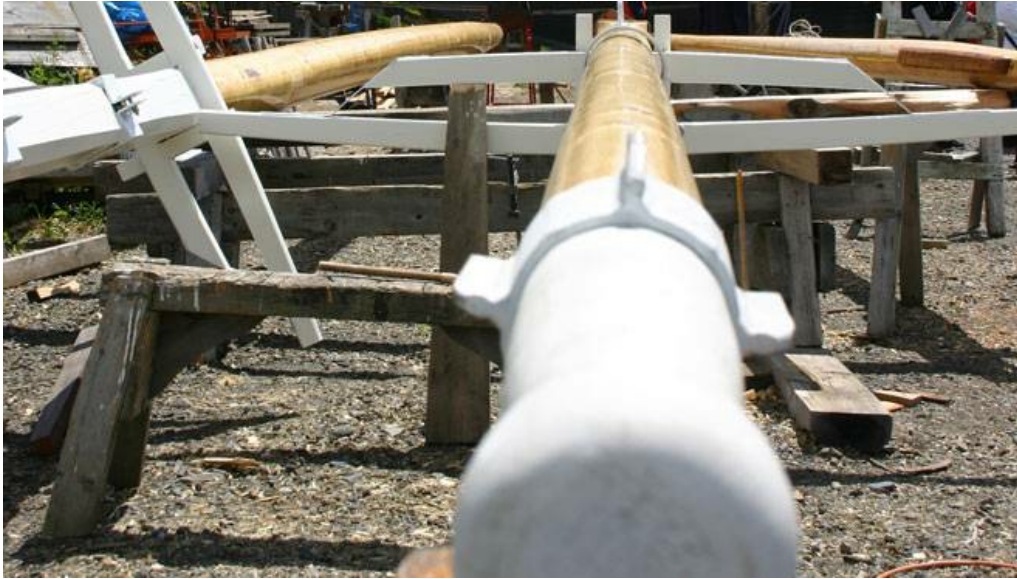
A mast is ready to be installed in one of two wooden schooners being built at The Dory Shop in Lunenburg. (BEVERLEY WARE / South Shore Bureau)
